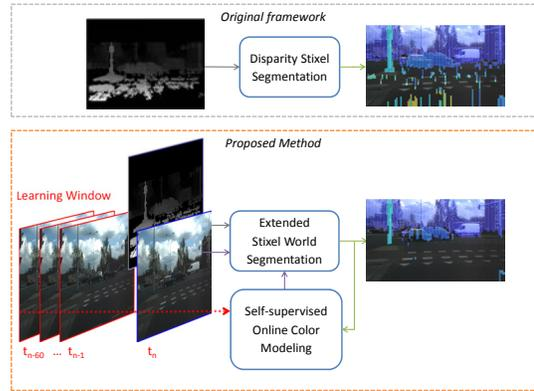
Fig. 2. The original stixel framework (top), relies on disparity images alone. In contrast, our proposed extension (bottom) exploits both disparity and color information.
