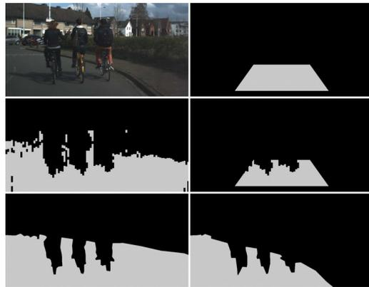
Fig. 3. Illustration of our *training mask* approach to acquire road samples. Top-left: input image; top right:  $TM_{prior}^g$ ; middle left: ground segmentation mask; middle right: intersection of the two,  $TM_t^g$ . The bottom row illustrates the different ground-truth annotations, with left *drivable surface* and right *road*.
