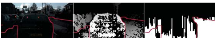
Fig.2: Left to right: dark input image, noisy disparity signal, corresponding weak labels for online training. Manual groundtruth in red.
