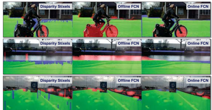
Fig.3: Left to right: Stixel World; offline trained FCN; online tuned FCN. Green: true free space; Red: missed obstacles; Blue: false obstacles
